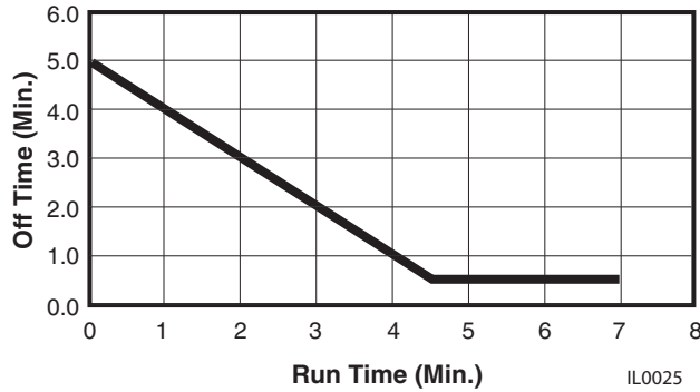
CP Water Pump Underload "Smart Reset"
