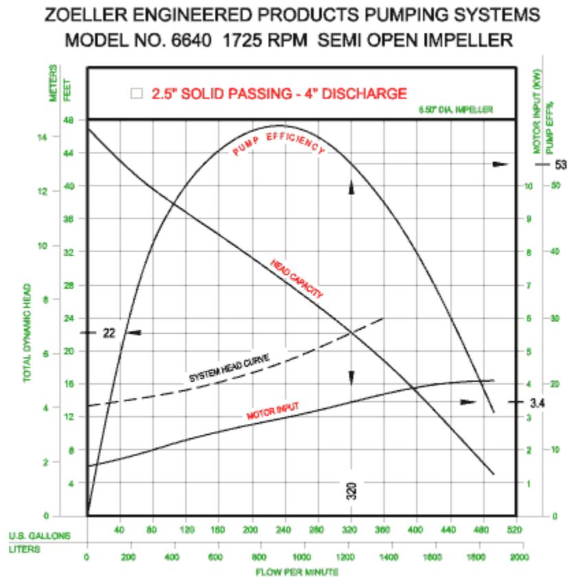
Each of the above items is calculated from the performance data obtained when testing a pump. The pump test can either be done at the factory or in the field with the appropriate equipment. Head, capacity, current, power input, and voltage are all items that are read by the test equipment. Power factor, motor efficiency, motor input horsepower (EHP), brake horsepower (BHP), hydraulic horsepower (WHP), total efficiency, and pump efficiency must be calculated or looked up in tables.
